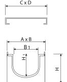
Channel made of high density polypropylene.
